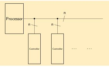
In most cases the n lines of the bus can be views as 3 busses: the address bus, the data bus and the control bus
